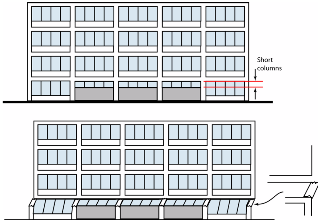
Figure 5-2 Elevation views of building with short columns between first and second floors. Upper sketch show the building in an unshaken state; lower sketch shows damage mechanism under earthquake lateral loading.
